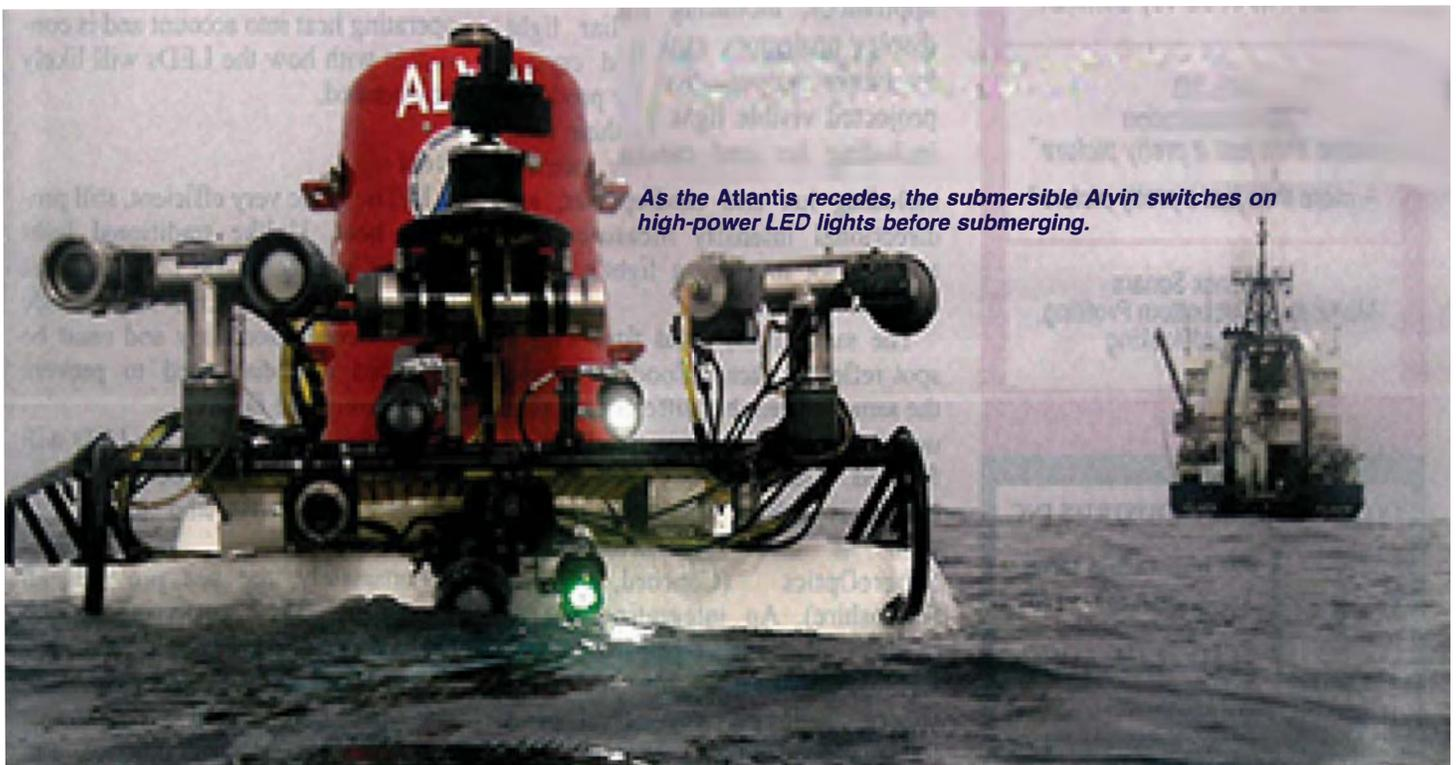
*As the Atlantis recedes, the submersible Alvin switches on high-power LED lights before submerging.*
